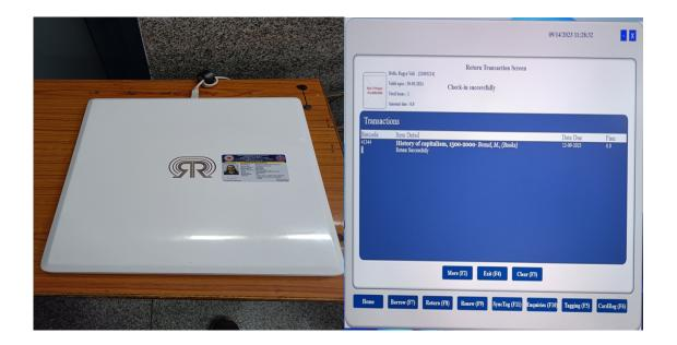
RFID Staff Station Reader is a staff assisted station on services such as loan, return, tagging, sorting and etc. The integrated reader features excellent tag read/write operation performance with a high identification rate. The staff puts the item on the reader and click on the view to display the information stored inside the tag.
